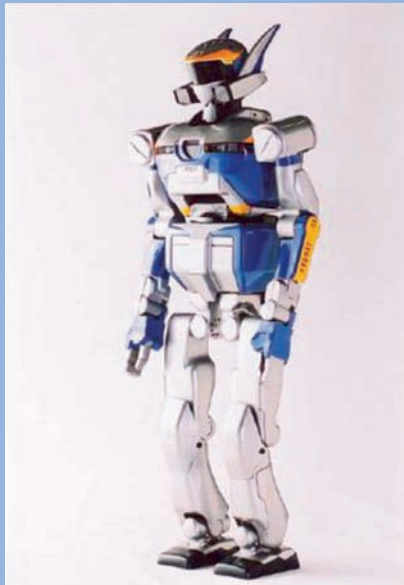
RESİM ALTI: HRP2 İnsansı Robot. Otuz serbestlik dereceli, Boy 154cm, ağırlık 58kg. Kawada Industries, ve Humanoid Research Group of National Institute of Advanced Industrial Science and Technology (AIST) (Japonya).
